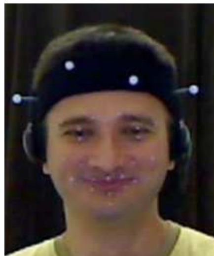
Figure 2: Infrared markers placed for facial motion tracking using OptiTrack
